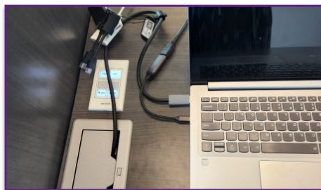
4 Connect Owl camera cable to laptop
